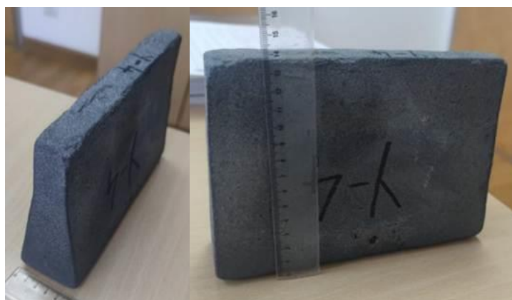
Figure 1. Initial Y block from which the samples were machined
