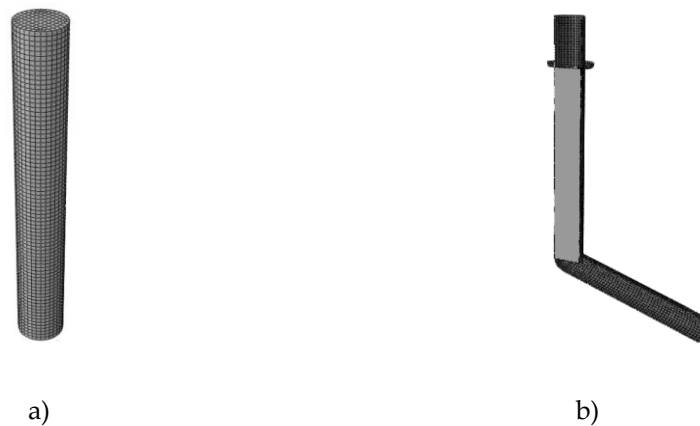
Figure 2: a) Workpiece after discretization, b) Workpiece, Punch, and channel assembly (section view) [18]
