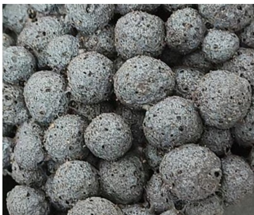
Figure 4. The photo of reduced laterite nickel ore leaching residue pellets
