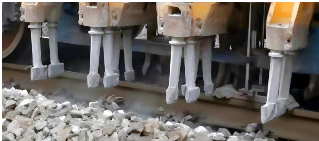
Figure 1. On-site photos of the tamping picks
